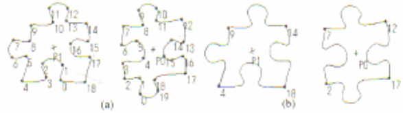
Fig. 6 (a) is the dominant points from the boundary curves in Fig. 4 (h), and (b) is the corner points detected from (a).
