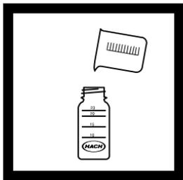
4. Fill the square mixing bottle to the 20-mL mark with sample water.
