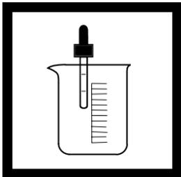
5. Rinse the plastic dropper several times with the sample water. If the sample is turbid, see instructions under *Sample Preparation for Testing Boiler Water or Other Turbid Waters (PO-19A)*. (The necessary apparatus is included in Kit PO-19A.)
