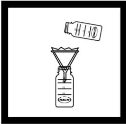
**5.** Pour the water sample into the filter paper and allow the sample to filter through. Test this clear water sample for phosphate.
