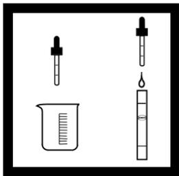
**6.** Fill the dropper to the first (0.5-mL) mark with the sample water. Put this water in the second viewing tube.
