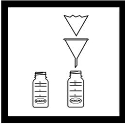
**4.** Place the funnel in the other square mixing bottle. Insert a folded filter into the funnel.
