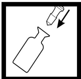
2. Incline the bottle slightly and insert the stopper with a quick thrust to avoid trapping air bubbles. If bubbles become trapped, discard the sample and repeat the test.
