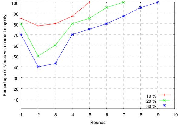
**Fig. 8: Percentage of nodes that compute the right decision for confidence levels lesser than or equal to 30 % threshold.**
