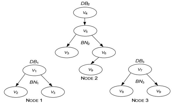
Fig. 1: A global database distributed at three nodes.
